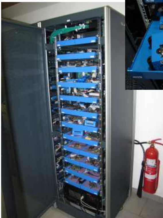
Test stand for automated regression testing of iSYSTEM tools connected to reference as well as custom targets
