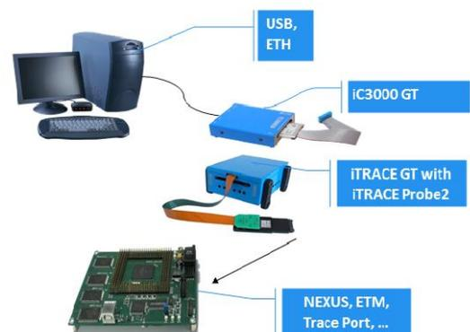
Figure 10: iC3000 with iTRACE GT and iTRACEProbe2
