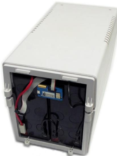
*Figure 1 UPS with iONE-BT debugger attached*
