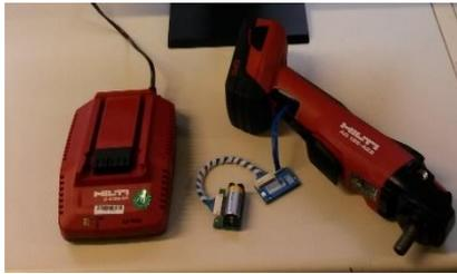
*Figure 7 iONE-BT being used within Hilti's embedded software test concept for corded and cordless electric tools*
