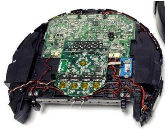
*Figure 2 Mobile Embedded System with iONE-BT debugger attached*
