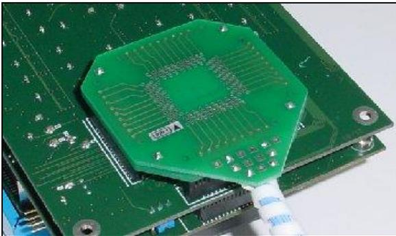
**Step 3:** Connect the POD via IA144P144TQ-W to the target.
