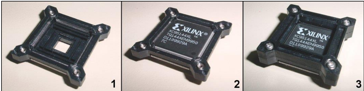
IA144YAM-SOLDER used to insert the CPU directly to the target
