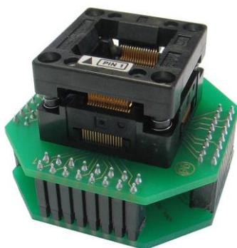
When the target is already adapted for the emulator connection through the IA64ATQ-SOLDER (soldered to the target PCB), the IA64ATQ-CPU allows testing the target application with the original microcontroller instead of the emulator.
