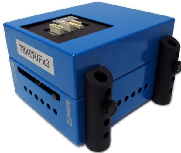
*IA100PODRL78F14 converter board assembled in the POD*
