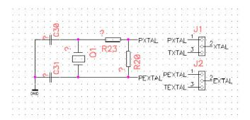
Jumpers J1 and J2 are used for clock source setting. When both jumpers are set to the position 1-2, the clock built on the Adapter is used and in this case, Q1, C30, C31, R20 and R23 must be populated. If the jumpers are set to 2-3, the clock from the target is used.
