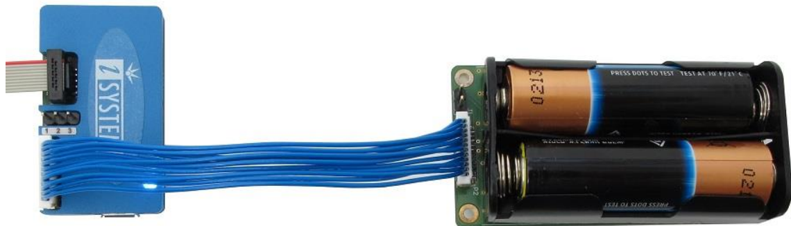
iONE-BT powered from the backup power supply
