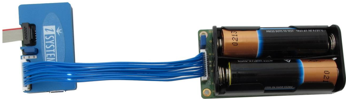
iONE-BT powered from the target with backup power supply
