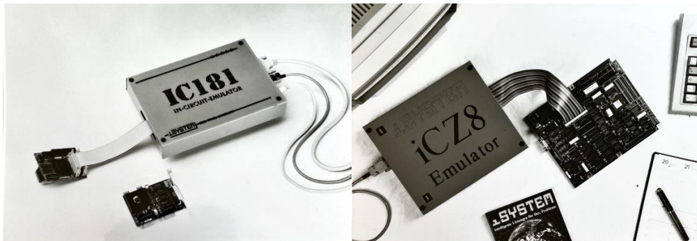
Figure 1: In-circuit emulation at the end of the 1980s
